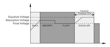
However, in Equalize stage, when battery equalized time is expired and battery voltage doesn't rise to battery equalization voltage point, the charge controller will extend the battery equalized time until battery voltage achieves battery equalization voltage, If battery voltage is still lower than battery equalization voltage when battery equalized timeout setting is over, the charge controller will stop equalization and return to float stage.
