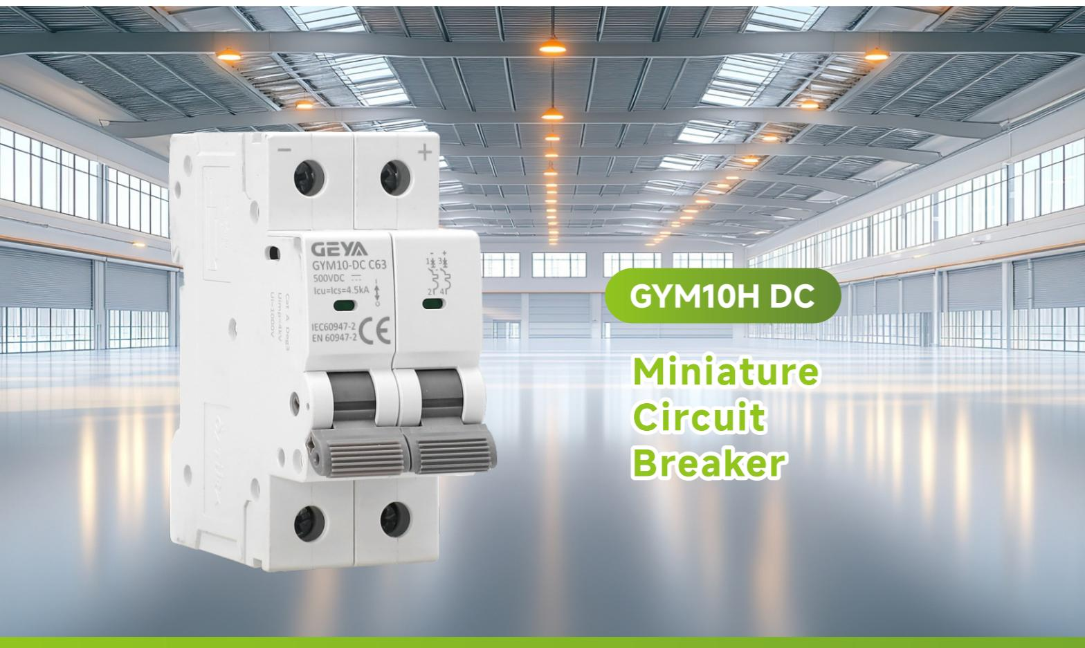
The GYM10H DC circuit breaker is designed for DC circuits with rated voltage up to 1000V and rated current up to 63A, providing overload and short-circuit protection, and can also be used for infrequent circuit switching operations.
