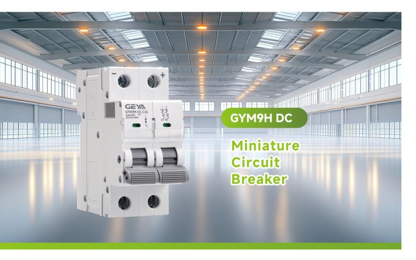
GYM9 DC Circuit Breaker is designed for DC circuits with a rated voltage up to 1000V and a rated current up to 63A. It provides overload and short-circuit protection and can also be used for infrequent switching operations of circuits. This circuit breaker is suitable for DC system applications, such as communications and photovoltaic (PV) systems. Compliance Standards: IEC/EN 60947-2 GB/T 14048.2
